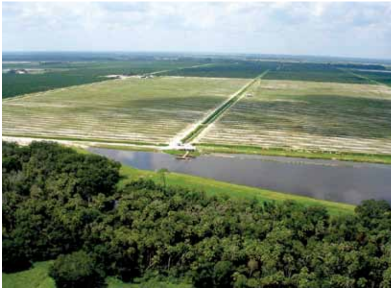
Aerial of the 15-acre tailwater recovery reservoir and pump station in the foreground of FARMS project H516 Hancock Grove, DeSoto Co. The reservoir provides offset of groundwater on approximately 700 acres of the entire 1,400 acre citrus grove.
